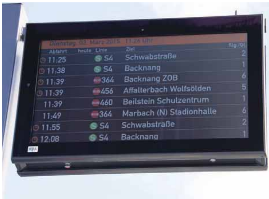
RTPI station and stop displays across the Stuttgart region
