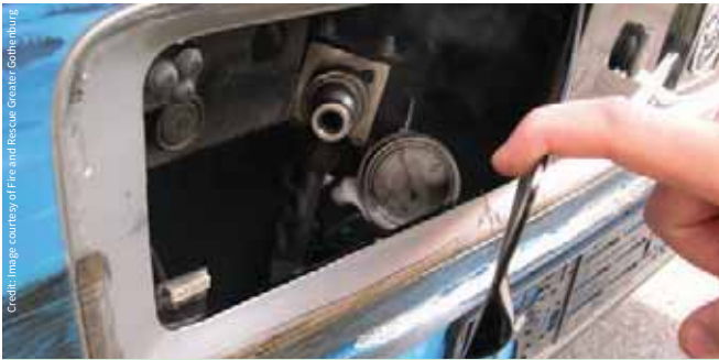
Leakage of gas from the manometer
