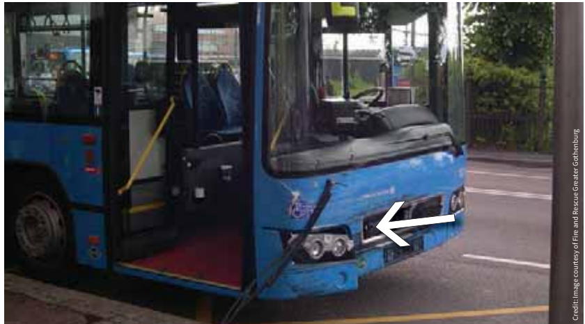
Image 1: A CNG bus involved in an accident; the arrow shows the position of its leakage
