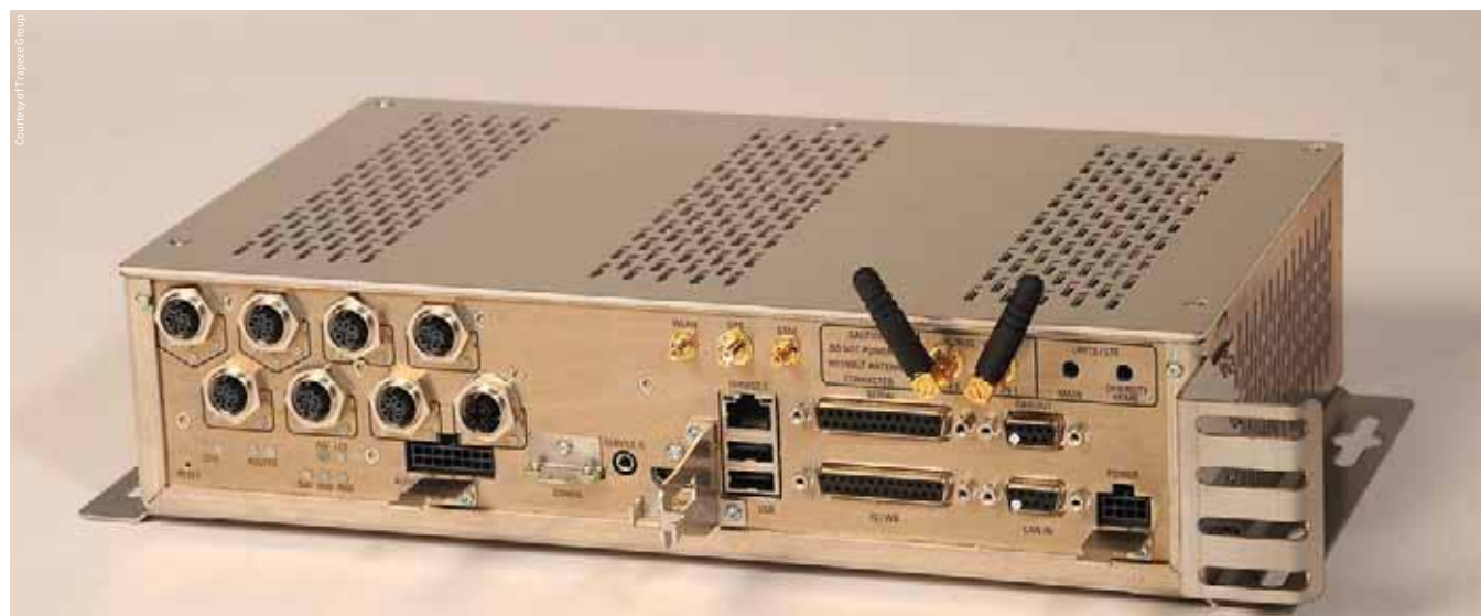
Making it all happen: the Intelligent Data Router (IDR) from Trapeze Group which is installed on each vehicle
